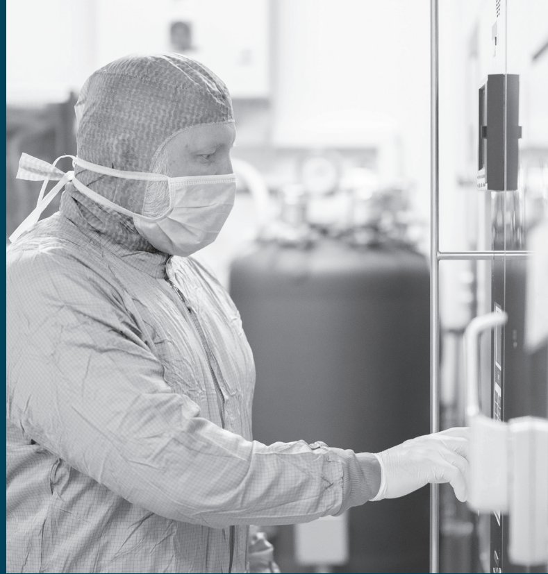
Operation of the freeze-drying system in the clean rooms of C+TBA in Krems on the Danube. Freeze drying is a gentle method of preserving bone grafts.
